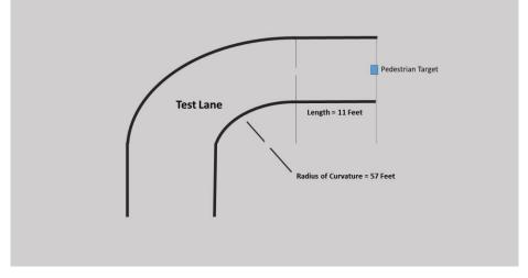
Figure 25: Illustration of test lane (not drawn to scale) Image Source: AAA
