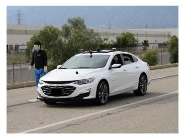
Figure 3: 2019 Chevrolet Malibu outfitted with measurement equipment Image Source: AAA
